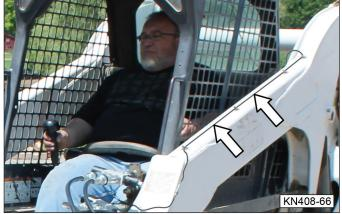
Mount the control button in the cab.
