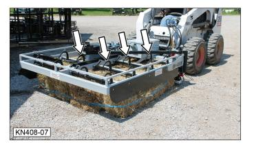
**Note:** In some cases, fully opening the squeeze arm without lifting the unit off of the bales, can cause the twine to break.
