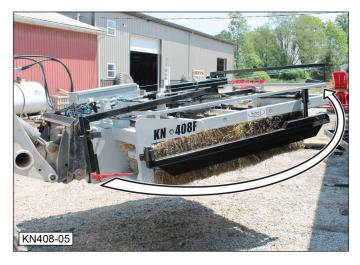
Continue to hold the "Twine Arm Forward" lever/control and once the twine arm needle threads the twine completely, the knotter assembly will automatically tie the twine. Do not release the lever/control while the knotter is in operation.
