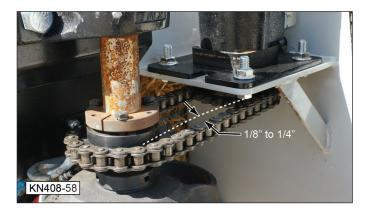
To adjust the tension on the chain, loosen four bolts (1) and adjust bolt (2) to achieve the proper chain tension.
