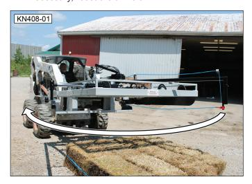
Position the unit over the bales. Driving slightly forward and to the right will condense the bales into a more compact grouping.
