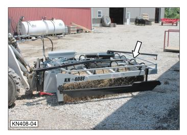
5. Press and hold the lever/control for the "Twine Arm Forward" circuit to extend the twine arm around the bales. Releasing the lever at any point in the operation will stop the movement.
