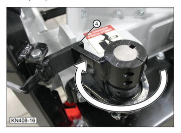
When the twine arm returns to its retracted position, the actuation plate releases the flow control valve and stops hydraulic oil flow to the motor. The motor stop plate (4), part of the twine arm, is also retracted. Since there is no hydraulic flow to the motor it is positioned for the next cycle.
