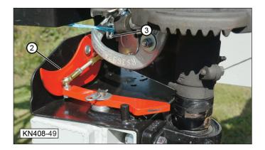
3. As the knotter cycles, cam (3) on the knotter shaft contacts and rotates rocker arm (4) causing tucker finger (2) to push the twine into the knotter.
