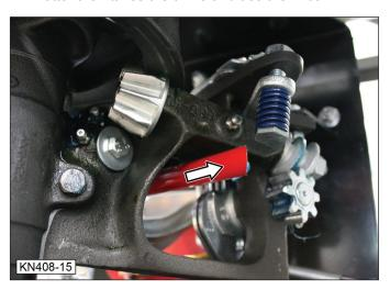
5. As the knotter assembly finishes tying the knot, the shaft has rotated and contacts knotter stop plate (4). This plate prevents the knotter from further rotation.
