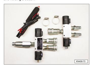
1. Connect two valves (5) into the hydraulic circuit ports.
