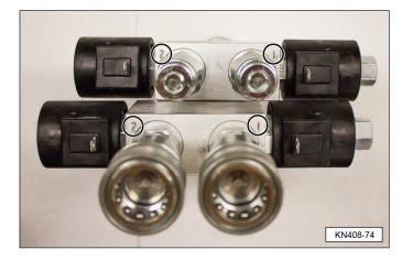
2. Connect the outlet (1) and inlet (2) hoses for the squeeze arm and bale hook circuit to the splitter valve ports marked number 1. Connect the outlet (3) and inlet (4) hoses for the swing arm and knotter circuit to to the splitter valve ports marked number 2.
