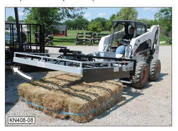
11. Press and hold the lever/control for the "Twine Arm Return" circuit until the twine arm returns to its retracted position and then release the lever/control. Releasing the lever at any point in the operation will stop the movement.
