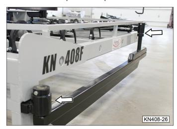
3. Lubricate two motor shaft bearings.
