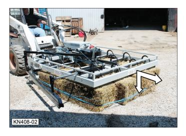
3. Press and hold the lever/control for the "Close Squeeze Arm" circuit. Releasing the lever at any point in the operation will stop the movement.
