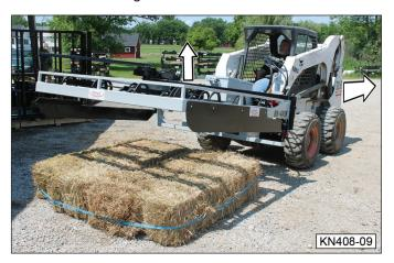
10. Once clear of the bales, activate the squeeze arm open circuit to open the squeeze arm.
