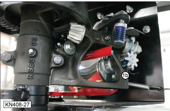
2. When tucker finger (2) is in the down position, as shown, bill hook finger (3) should also be pointed down.
