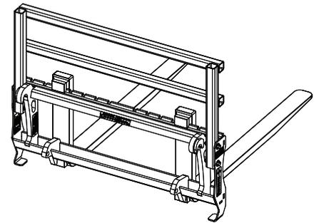
The Norden Euro Pallet Forks are an attachment that mounts to a loader or a tractor equipped with a loader having similar mounting capabilities. It is designed to move heavy pallet loads with ease.
