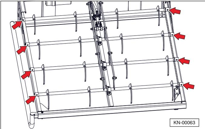
Oil the eight center bar linkage pivot points and the four hook bar center brackets weekly.
