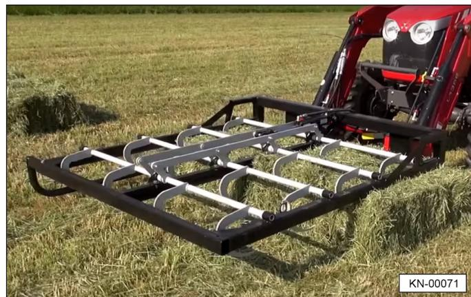
3. Move to the next row of four bales, position the crowd bar against the right side of the row of bales, lower the Grabber onto the bales, and release the bale hooks.
