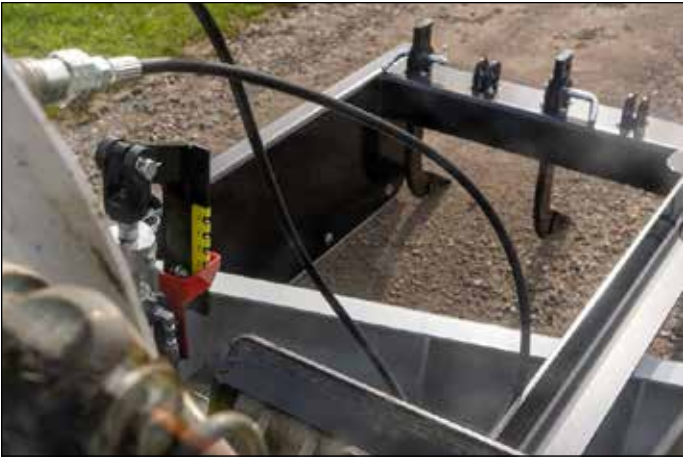
Left-hand — "Grade Height" adjustment (0 through 4).
