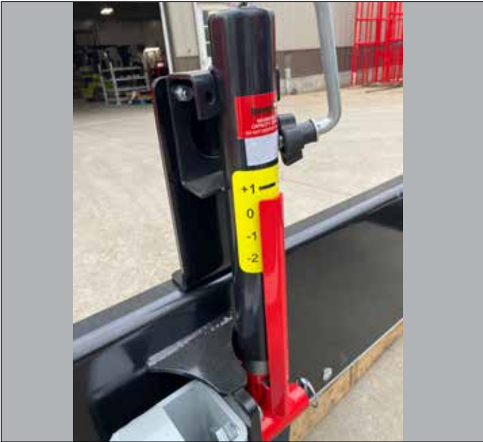
Right-hand — "Cutting Height" adjustment (+1 through -2).
