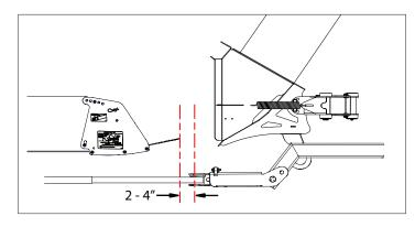
4. Insert hitch pin, place hitch in to retracted position.
