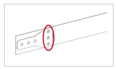
14. Use a 3/8" leather punch (recommended) or a 7/16" drill to make three holes through the belt at the marked locations.
