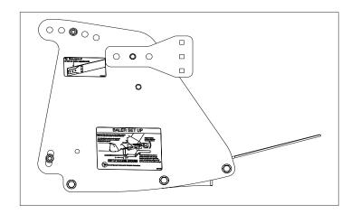
12. Hold the belt on the outside of the large end plate, pull the belt snug and mark a line on the belt even with the back end of the plate.
