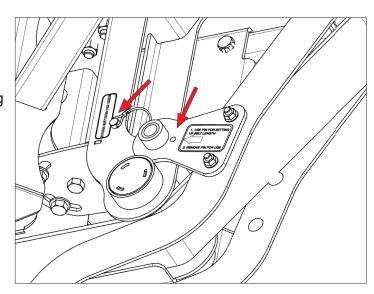
17. Ensure that the belt tensioner assembly is square with the belt by adjusting the angle of the belt tensioner assembly at its mounting point on the base chute.
