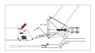
6. Tighten the four carriage bolts on the sides of the chamber extension first, then the six flange bolts on the bottom. Install Lighting Cable using 5/16" bolts, washers and nylock nuts.
