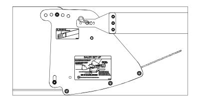
TIP: If your accumulator is equipped with a winch on the upright, hook the winch to the tensioner using the same slot as the spring, and crank to relieve tension. After attaching belt plates, loosen winch cable and remove from the Tensioner.
