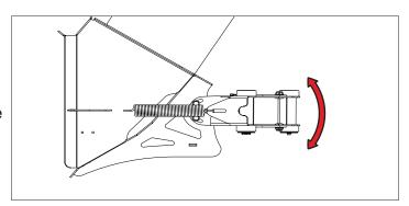
18. Fasten the belt plate to the previously selected pin on the side of the Chamber Extension.
