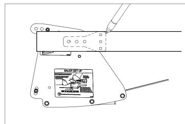
13. Place the belt on a flat surface. Remove the large end plate from the pin and place it on the belt with the back edge on the previously marked line. Mark the hole locations.
