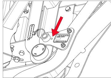
11. On the driver side, temporarily mount the large end plate on the appropriate pin using the same hole as the other side.
