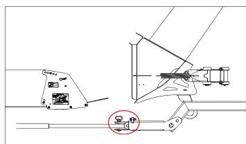
5. Select the hole that aligns the bottom plate of the bale chamber extension to a point 8-10" back from the base chute bottom edge as shown. This can be fine tuned later if needed to achieve optimum results.
