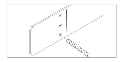
15. Install the belt end plates using three 3/8 x 1" carriage bolts and flange nuts. Position the large end plate on the inside (nearest to the bale chamber). Remove the excess belt length leaving about 6" for future adjustments.
