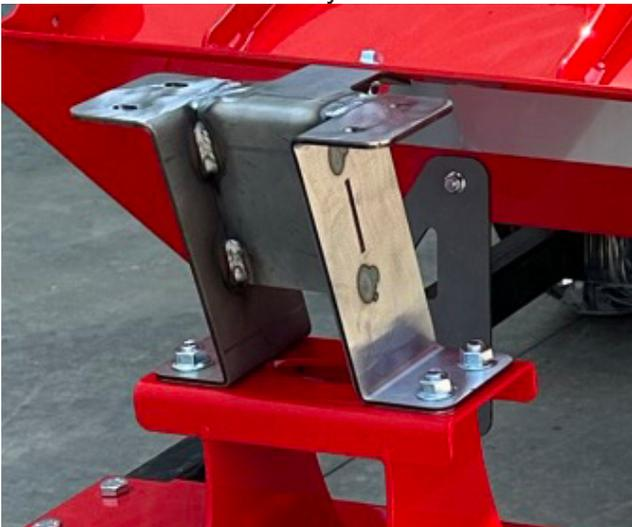
4. Remove the shipping brackets holding the front of the bed to the reach poles.
