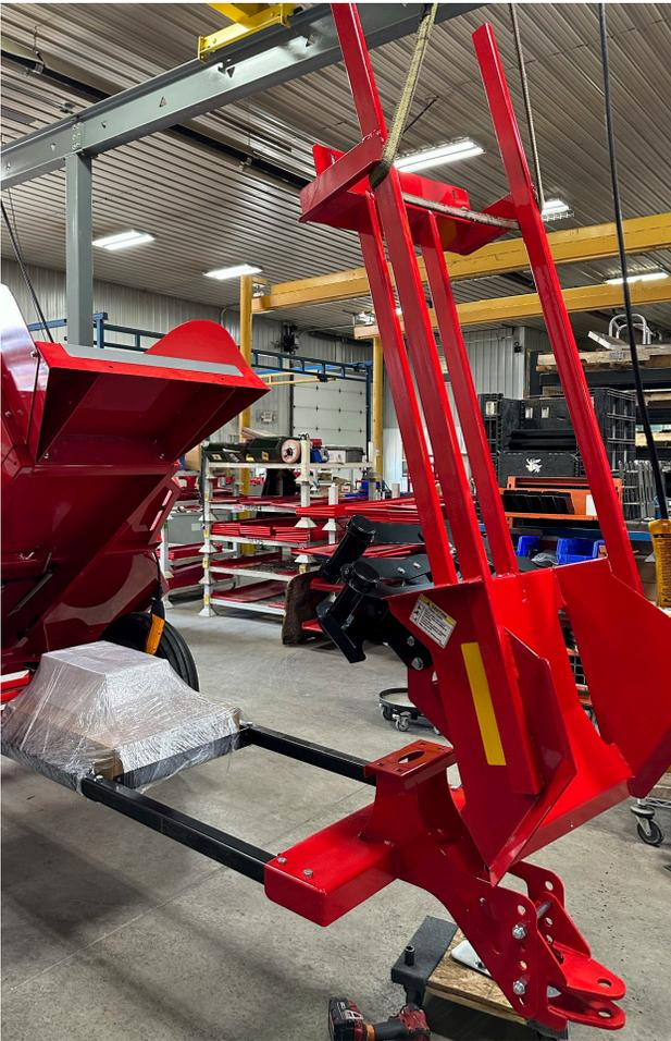
9. Set the chute assembly onto the frame, line up the bolt holes at the bottom.
