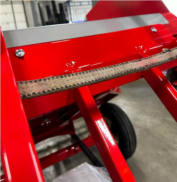
13. Tighten the (4) bolts at the bottom of the chute you placed in step 9.
