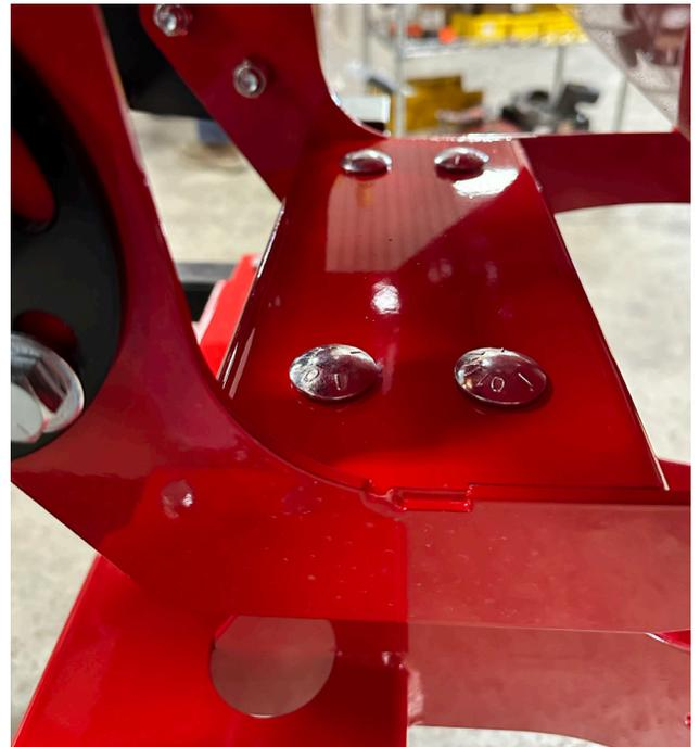
11. The top of the chute is fastened to the accumulator with two 3/8" x 1" Carriage bolts. Use an alignment tool to position the chute and bed to allow placement of first bolt.
